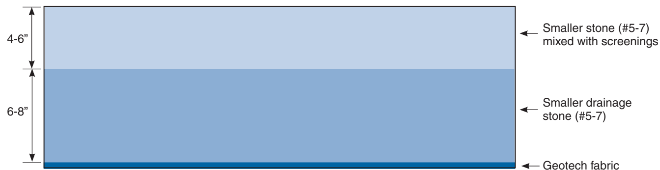
Figure 2. Drylot Pad Footing
