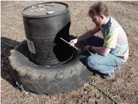
Photo 2. The threaded rod goes through the wall of the barrel into the inside of the tire
